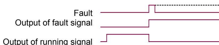
Figure 6.12 Sequence of fault signal
