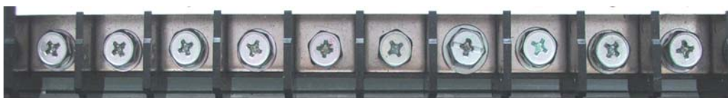
Figure 4.6 Main circuit terminals for 30kW Inverters
