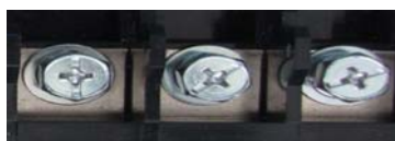
Figure 4.5 Main circuit terminals for 18.5kW/22kW Inverters
